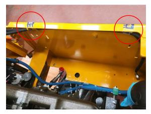
10.2. Using a suitable lifting device pick up and lower tank carefully into chassis front end first (35kg).
