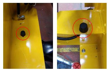
7.9. Remove mounting brackets and rubber buffers from chassis 9 & 10T machines. Discard.
