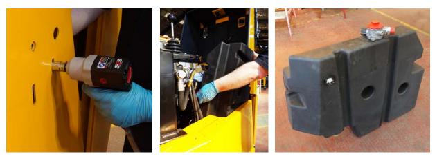
7.8. Remove the two rubber buffers from chassis 5 & 6T machines. Discard.
