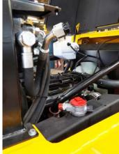
5.4. Remove LH side cross brace fixings (2 x M10 bolts).
